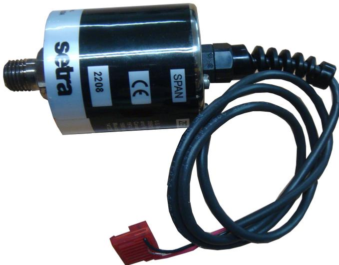
Fig. 2.6 Photograph of pressure gauge.
