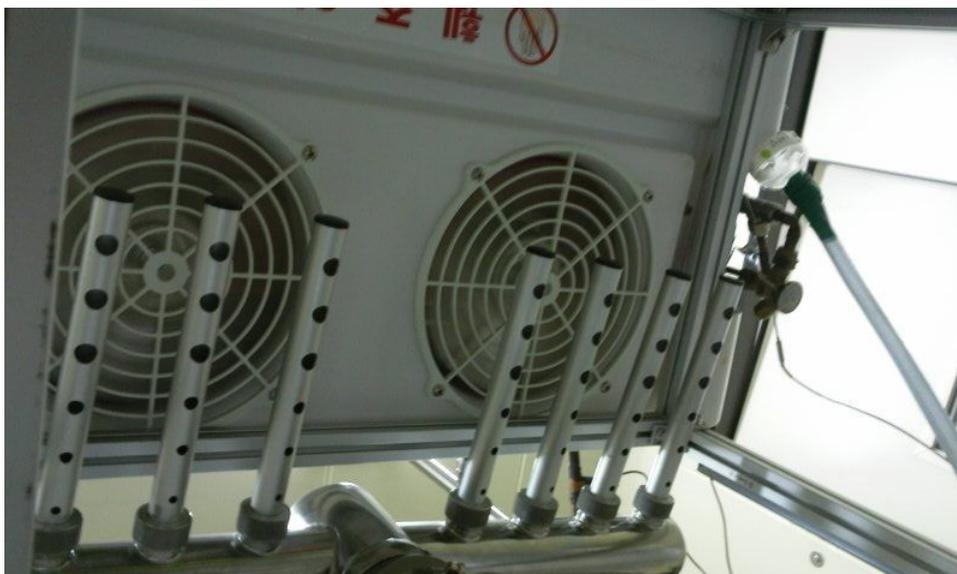
Fig. 2.10 Air sampler of indoor side.
