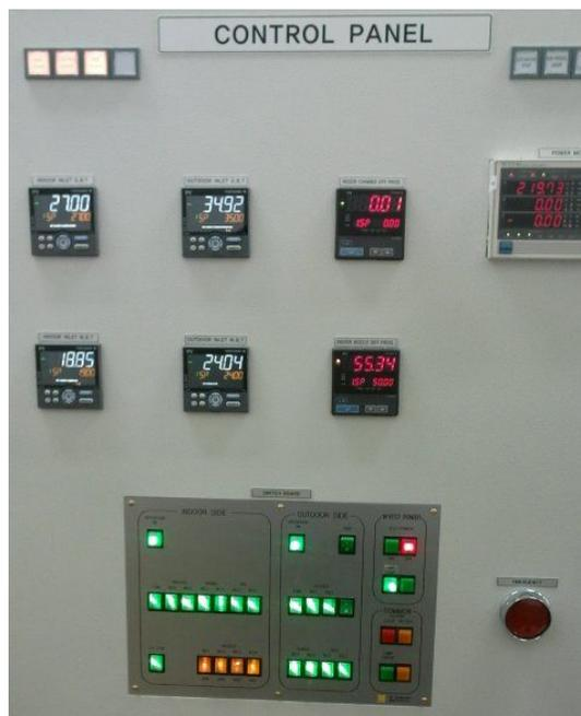
Fig. 2.4 Control panel of psychrometric chamber.
