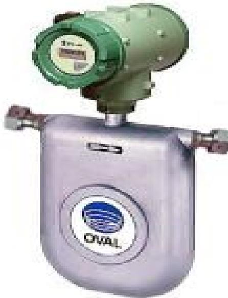
Fig. 2.9 Photograph of mass flow meter.
