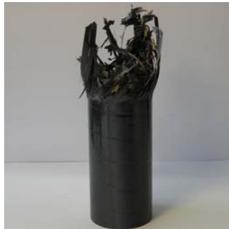
Photo. 22 Shape of Collapse CFRP Circular member, [-15/+15]_4 (Static, 15^\circ fiber orientation angle, Impact Energy 419.44J)
