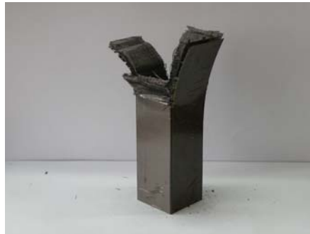
Photo. 54 Shape of Collapse CFRP Square member, [90]_8 (Static, 90^\circ fiber orientation angle, Impact Energy 274.4J)
