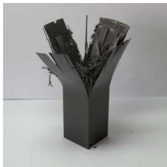
Photo. 32 Shape of Collapse CFRP Square member with orientation angle 0^\circ (Impact Energy 372.4J, Interface number 4)
