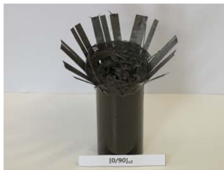
Photo. 5 Shape of Collapse CFRP Circular member with orientation angle 0^\circ (Impact Energy 611.52J, Interface number 4)
