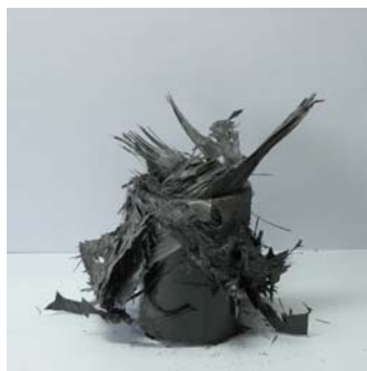
Photo. 23 Shape of Collapse CFRP Circular member, [-45/+45]_4 (Static, 45^\circ fiber orientation angle, Impact Energy 611.52J)
