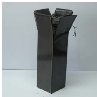
Photo. 31 Shape of Collapse CFRP Square member with orientation angle 0^\circ (Impact Energy 223.44J, Interface number 2)
