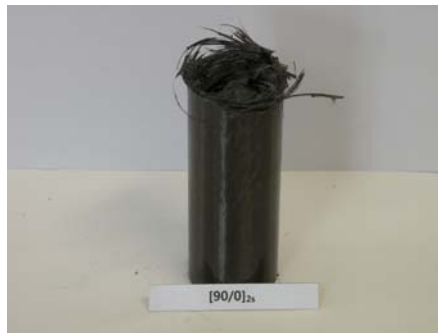
Photo. 19 Shape of Collapse CFRP Circular member with orientation angle 90^\circ (Impact Energy 419.44J, Interface number 6)
