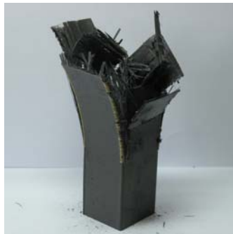
Photo. 46 Shape of Collapse CFRP Square member with orientation angle 90^\circ (Impact Energy 223.44J, Interface number 6)
