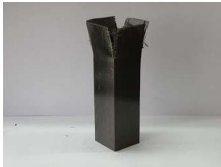
Photo. 52 Shape of Collapse CFRP Square member, [-45/+45]_4 (Static, 45^\circ fiber orientation angle, Impact Energy 223.44J)
