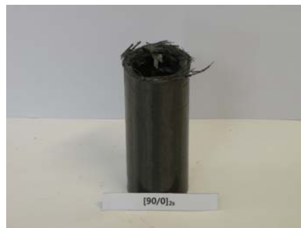
Photo. 18 Shape of Collapse CFRP Circular member with orientation angle 90^\circ (Impact Energy 529.20J, Interface number 6)
