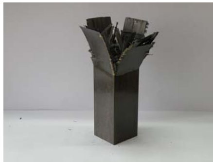
Photo. 50 Shape of Collapse CFRP Square member, [-45/+45]_4 (Static, 45^\circ fiber orientation angle, Impact Energy 372.4J)
