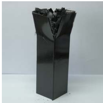
Photo. 36 Shape of Collapse CFRP Square member with orientation angle 0^\circ (Impact Energy 274.4J, Interface number 6)
