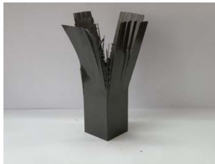
Photo. 48 Shape of Collapse CFRP Square member, [-15/+15]_4 (Static, 15^\circ fiber orientation angle, Impact Energy 274.4J)
