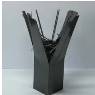
Photo. 37 Shape of Collapse CFRP Square member with orientation angle 0^\circ (Impact Energy 223.44J, Interface number 6)
