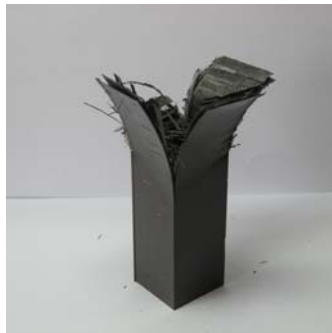
Photo. 44 Shape of Collapse CFRP Square member with orientation angle 90^\circ (Impact Energy 372.4J, Interface number 6)
