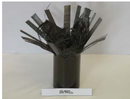
Photo. 8 Shape of Collapse CFRP Circular member with orientation angle 0^\circ (Impact Energy 611.52J, Interface number 6)
