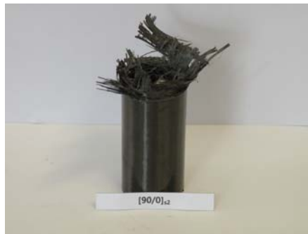
Photo. 14 Shape of Collapse CFRP Circular member with orientation angle 90^\circ (Impact Energy 611.52J, Interface number 4)
