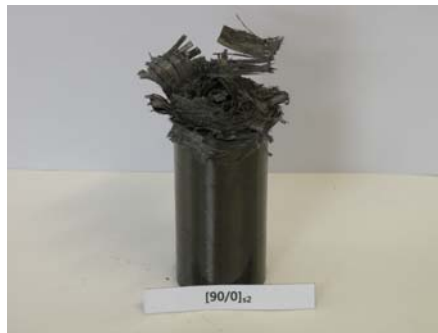
Photo. 16 Shape of Collapse CFRP Circular member with orientation angle 90^\circ (Impact Energy 419.44J, Interface number 4)
