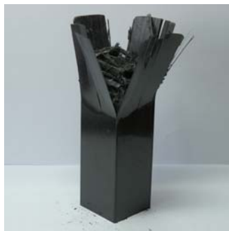
Photo. 39 Shape of Collapse CFRP Square member with orientation angle 90^\circ (Impact Energy 274.4J, Interface number 2)
