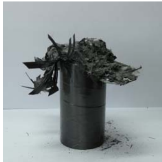
Photo. 24 Shape of Collapse CFRP Circular member, [-45/+45]_4 (Static, 45^\circ fiber orientation angle, Impact Energy 529.2J)
