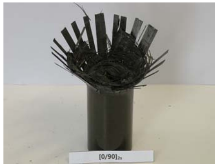
Photo. 9 Shape of Collapse CFRP Circular member with orientation angle 0^\circ (Impact Energy 529.20J, Interface number 6)
