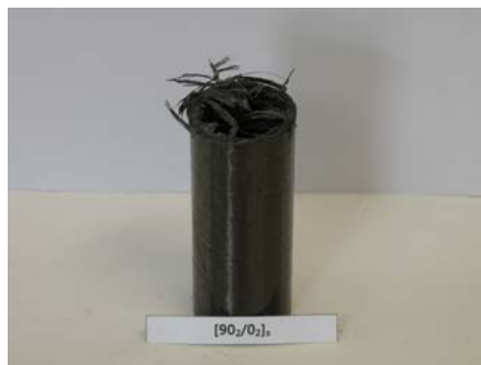
Photo. 12 Shape of Collapse CFRP Circular member with orientation angle 90^\circ (Impact Energy 529.20J, Interface number 2)
