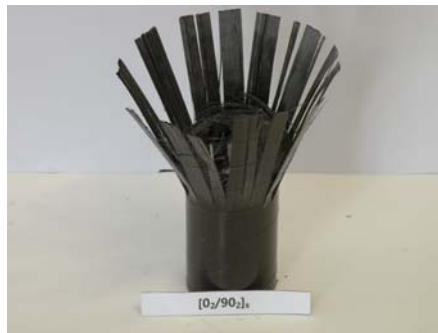
Photo. 4 Shape of Collapse CFRP Circular member with orientation angle 0^\circ (Impact Energy 419.44J, Interface number 2)
