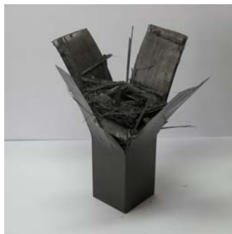
Photo. 35 Shape of Collapse CFRP Square member with orientation angle 0^\circ (Impact Energy 372.4J, Interface number 6)
