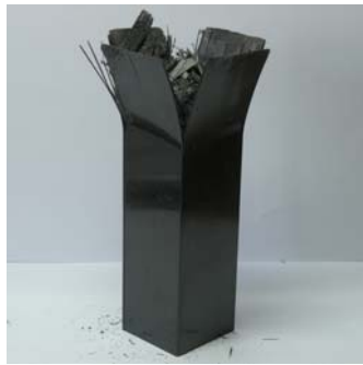
Photo. 45 Shape of Collapse CFRP Square member with orientation angle 90^\circ (Impact Energy 274.4J, Interface number 6)
