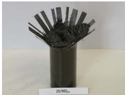
Photo. 10 Shape of Collapse CFRP Circular member with orientation angle 0^\circ (Impact Energy 419.44J, Interface number 6)
