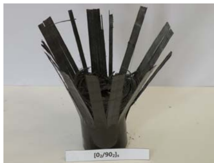
Photo. 3 Shape of Collapse CFRP Circular member with orientation angle 0^\circ (Impact Energy 529.20J, Interface number 2)
