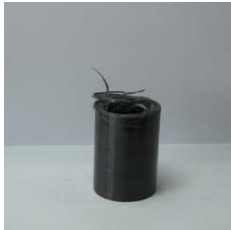
Photo. 26 Shape of Collapse CFRP Circular member, [90]_8 (Static, 90^\circ fiber orientation angle, Impact Energy 611.52J)
