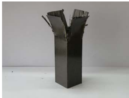
Photo. 51 Shape of Collapse CFRP Square member, [-45/+45]_4 (Static, 45^\circ fiber orientation angle, Impact Energy 274.4J)
