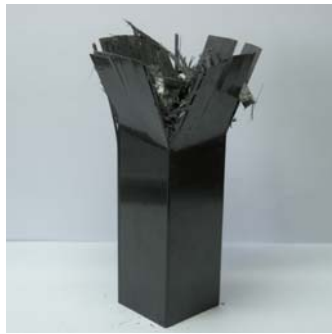
Photo. 34 Shape of Collapse CFRP Square member with orientation angle 0^\circ (Impact Energy 223.44J, Interface number 4)
