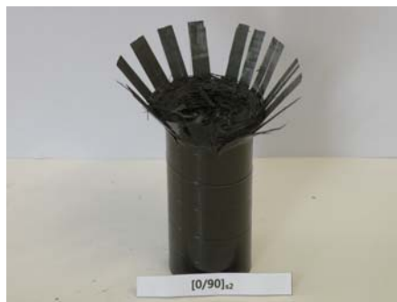
Photo. 6 Shape of Collapse CFRP Circular member with orientation angle 0^\circ (Impact Energy 529.20J, Interface number 4)
