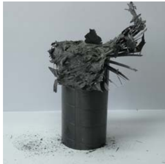
Photo. 25 Shape of Collapse CFRP Circular member, [-45/+45]_4 (Static, 45^\circ fiber orientation angle, Impact Energy 419.44J)
