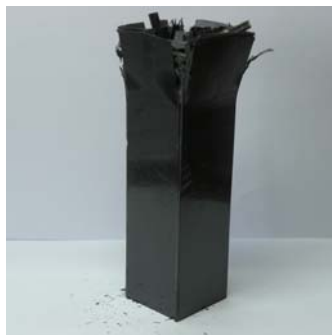
Photo. 40 Shape of Collapse CFRP Square member with orientation angle 90^\circ (Impact Energy 223.44J, Interface number 2)
