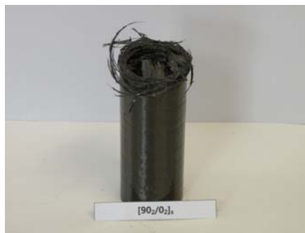
Photo. 13 Shape of Collapse CFRP Circular member with orientation angle 90^\circ (Impact Energy 419.44J, Interface number 2)
