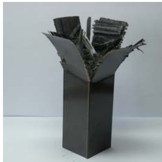
Photo. 30 Shape of Collapse CFRP Square member with orientation angle 0^\circ (Impact Energy 274.4J, Interface number 2)
