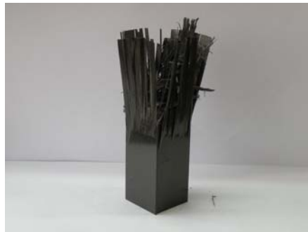
Photo. 47 Shape of Collapse CFRP Square member, [-15/+15]_4 (Static, 15^\circ fiber orientation angle, Impact Energy 372.4J)
