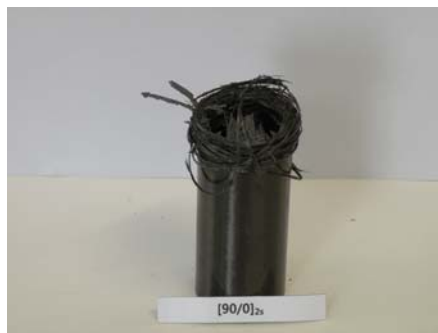
Photo. 17 Shape of Collapse CFRP Circular member with orientation angle 90^\circ (Impact Energy 611.52J, Interface number 6)
