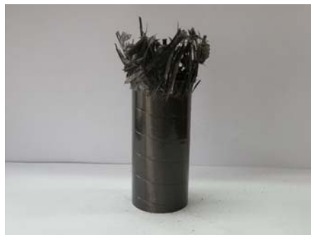
Photo. 21 Shape of Collapse CFRP Circular member, [-15/+15]_4 (Static, 15^\circ fiber orientation angle, Impact Energy 529.2J)
