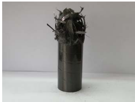
Photo. 20 Shape of Collapse CFRP Circular member, [-15/+15]_4 (Static, 15^\circ fiber orientation angle, Impact Energy 611.52J)
