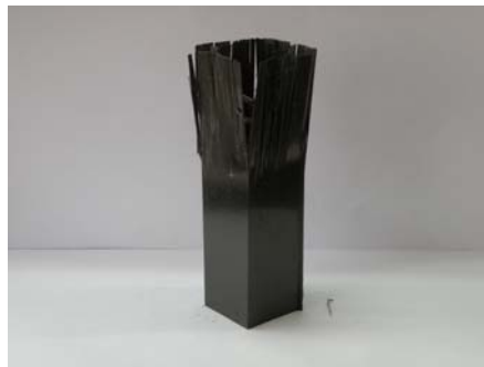
Photo. 59 Shape of Collapse CFRP Square member, [-15/+15]_4 (Static, 15^\circ fiber orientation angle, Impact Energy 223.44J)
