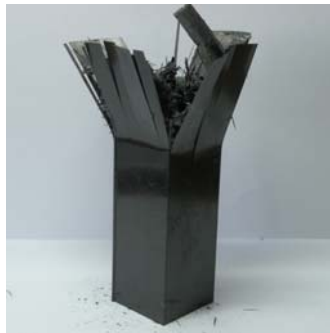
Photo. 43 Shape of Collapse CFRP Square member with orientation angle 90^\circ (Impact Energy 223.44J, Interface number 4)
