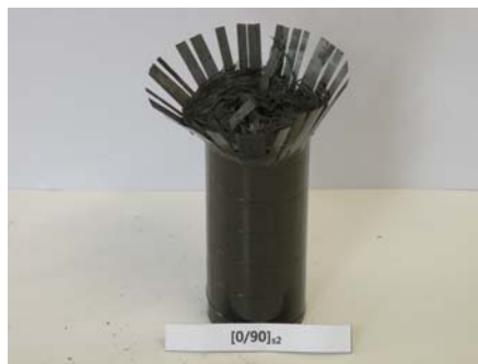
Photo. 7 Shape of Collapse CFRP Circular member with orientation angle 0^\circ (Impact Energy 419.44J, Interface number 4)
