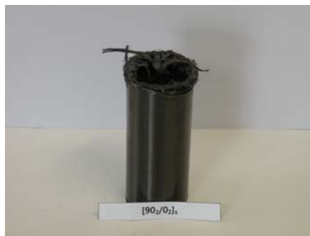
Photo. 11 Shape of Collapse CFRP Circular member with orientation angle 90^\circ (Impact Energy 611.52J, Interface number 2)
