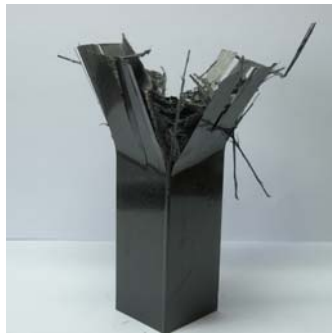
Photo. 33 Shape of Collapse CFRP Square member with orientation angle 0^\circ (Impact Energy 274.4J, Interface number 4)
