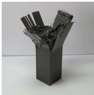
Photo. 29 Shape of Collapse CFRP Square member with orientation angle 0^\circ (Impact Energy 372.4J, Interface number 2)
