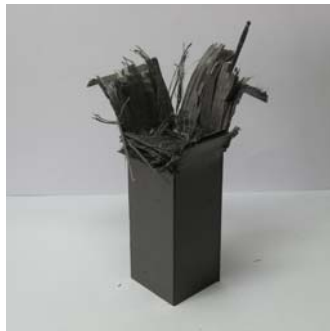
Photo. 38 Shape of Collapse CFRP Square member with orientation angle 90^\circ (Impact Energy 372.4J, Interface number 2)
