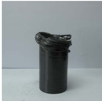
Photo. 28 Shape of Collapse CFRP Circular member, [90]_8 (Static, 90^\circ fiber orientation angle, Impact Energy 419.44J)
