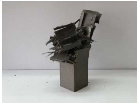
Photo. 53 Shape of Collapse CFRP Square member, [90]_s (Static, 90^\circ fiber orientation angle, Impact Energy 372.4J)
