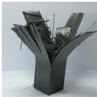
Photo. 42 Shape of Collapse CFRP Square member with orientation angle 90^\circ (Impact Energy 274.4J, Interface number 4)
