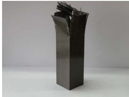
Photo. 55 Shape of Collapse CFRP Square member, [90]_8 (Static, 90^\circ fiber orientation angle, Impact Energy 223.44J)
