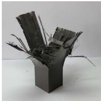
Photo. 41 Shape of Collapse CFRP Square member with orientation angle 90^\circ (Impact Energy 372.4J, Interface number 4)
