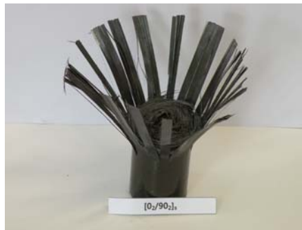
Photo. 2 Shape of Collapse CFRP Circular member with orientation angle 0^\circ (Impact Energy 611.52J, Interface number 2)
