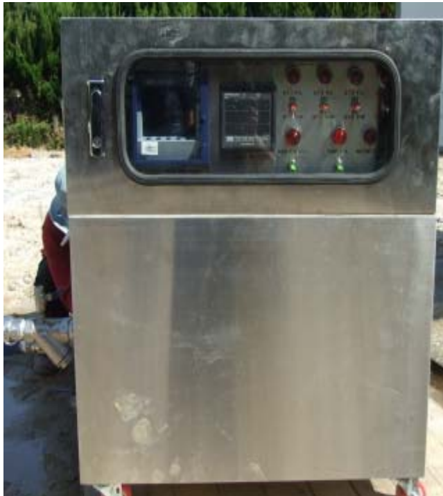
Photo. 1 In-situ ground effective thermal conductivity test unit
