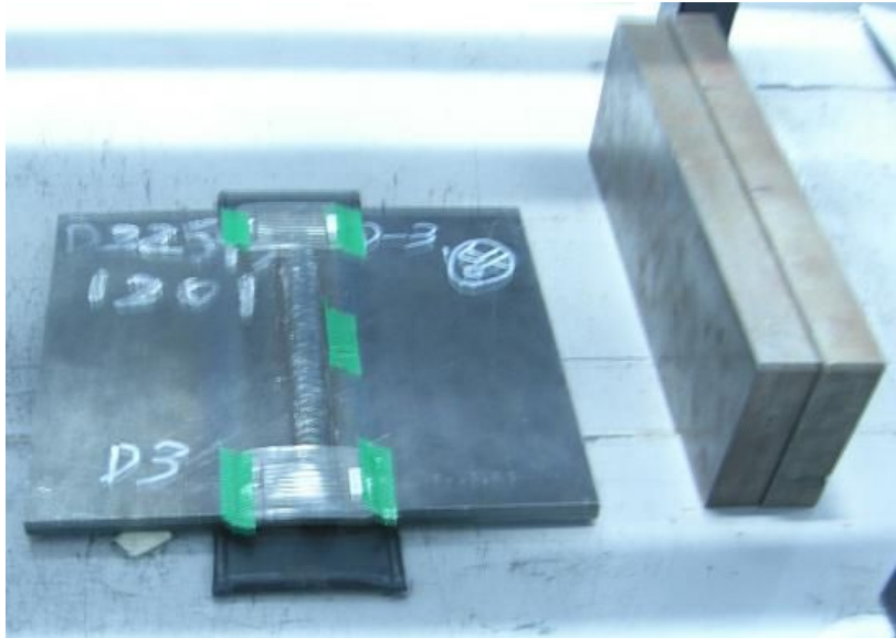
Fig. 3-19. X-ray Radiographic inspection of ATOS 80 welding specimen
