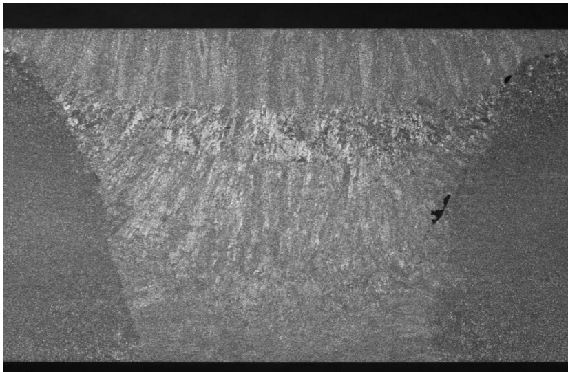
Fig. 3-16. Welding macro structure
