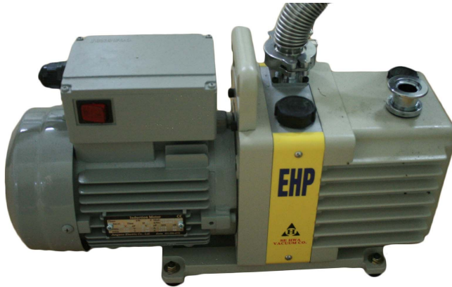
Fig. 2.28 Photograph of the vacuum pump.
