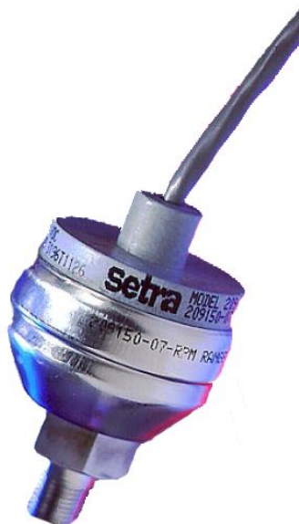
Fig. 2.16 Photograph of the pressure gauge(C209).
