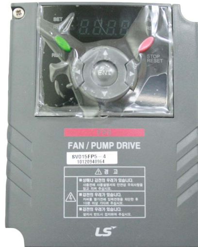
Fig. 2.27 Photograph of the inverter.
