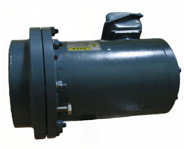
Fig. 2.25 Photograph of a solution pump.
