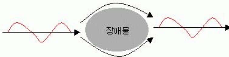
Fig 5. Diffraction of electromagnetic waves by an obstacle
