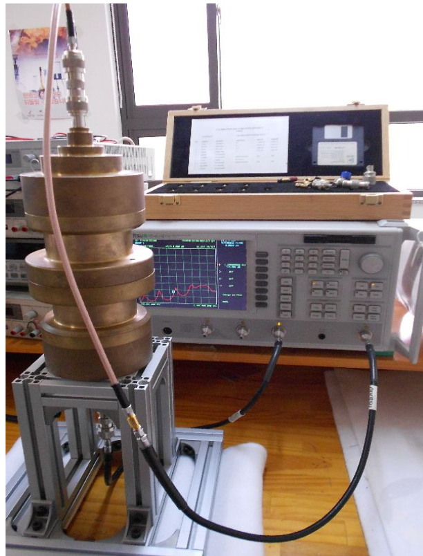
Fig. 11 Experimental set-up electromagnetic compatibility test system
