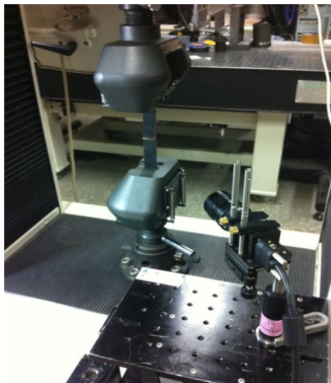
Fig.3-4 Measurement of volume by CCD Camera
