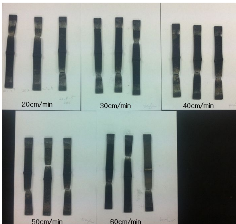
Fig. 4-2 Welded Specimen result by tensile speed
