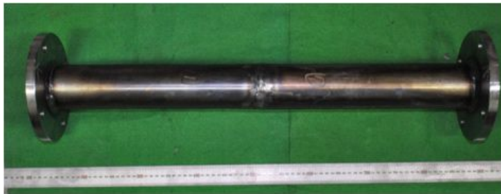
Fig. 3-11 2.5 inch pipe of ASTM A106 Gr.B material (700mm)
