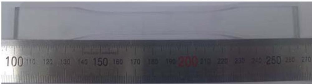
Fig. 23 Manufactured specimen for high temperature tensile test
