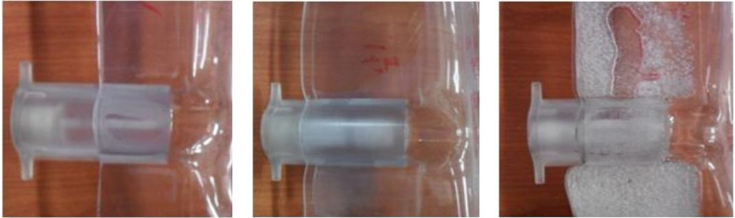
(a) Welding temperature = 155 °C (b) Welding temperature = 165 °C (c) Welding temperature = 175 °C
