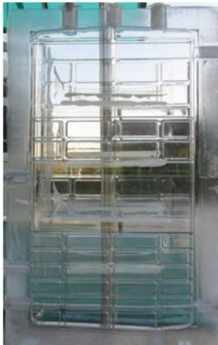
Fig. 57 Unified flat panel photobioreactor case via thermal welding process
