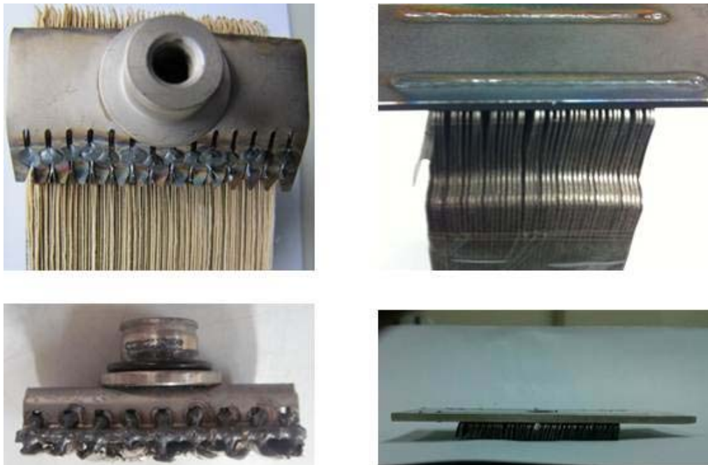
Fig. 4.35 Comparison of Argon TIG welding and laser welding
