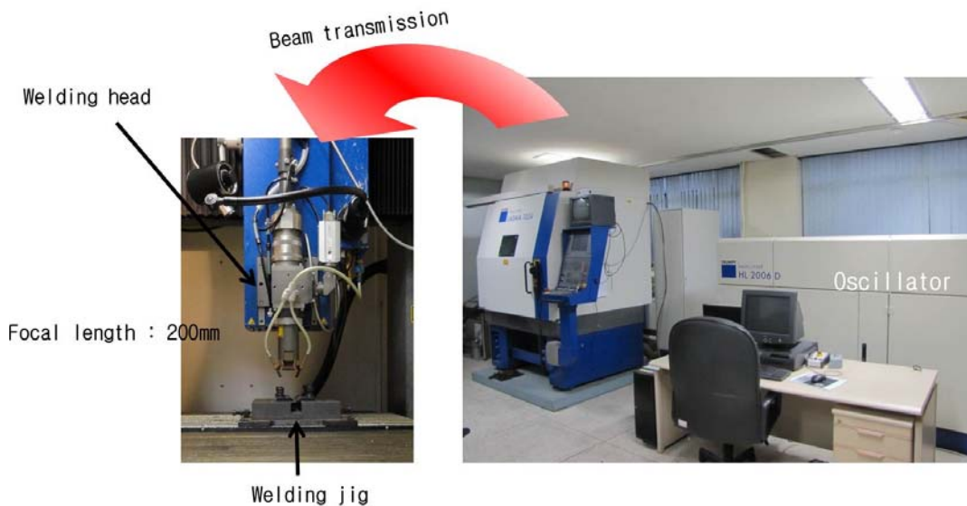
Fig. 3.3 Laser oscillator and optic head of welding processing
