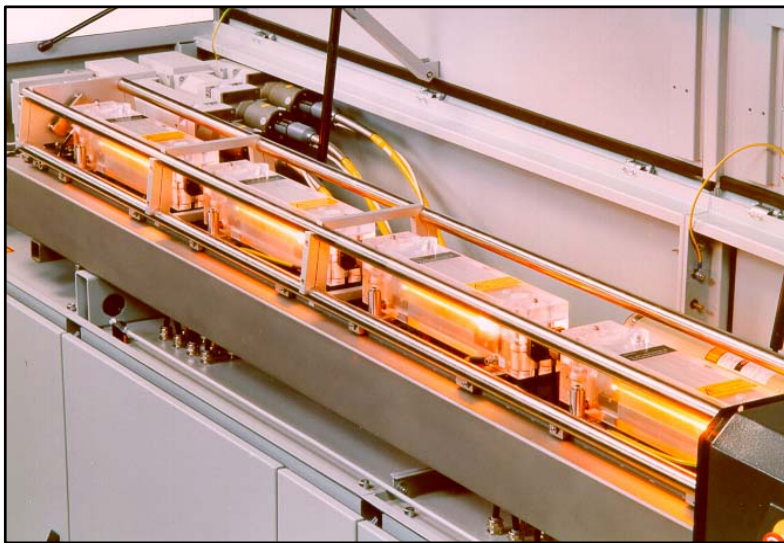
Fig. 2.1 High laser power is obtained by mounting several cavities in line(CW Nd:YAG laser)
