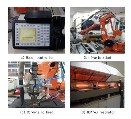
Fig. 3.3 Laser welding system
