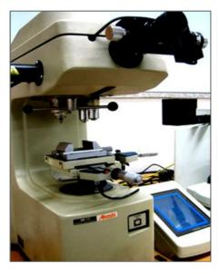
Fig. 3.9 Micro vickers hardness tester
