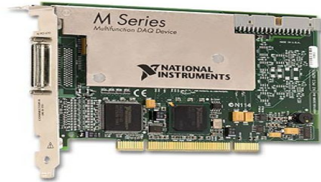
Fig. 3-12 Photo of high speed multifunction data acquisition
