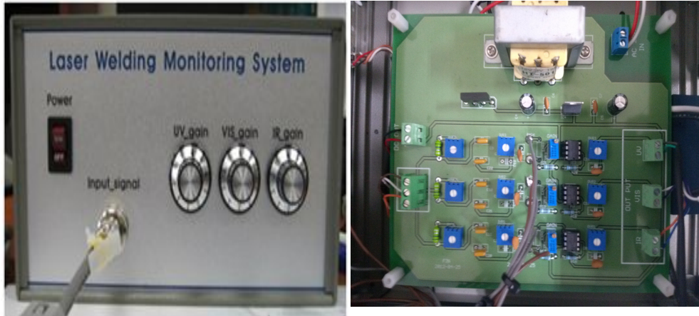
Fig. 3-11 Integrated monitoring system
