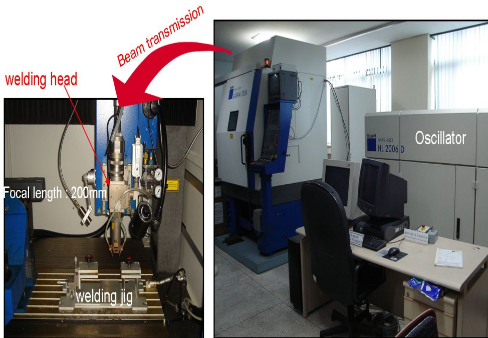
Fig. 3-2 Laser oscillator and optic head of welding processing
