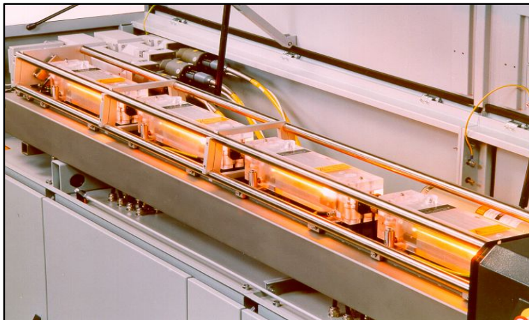
Fig. 3-1 High laser power is obtained by mounting several cavities in line(Continuous wave Nd:YAG laser)
