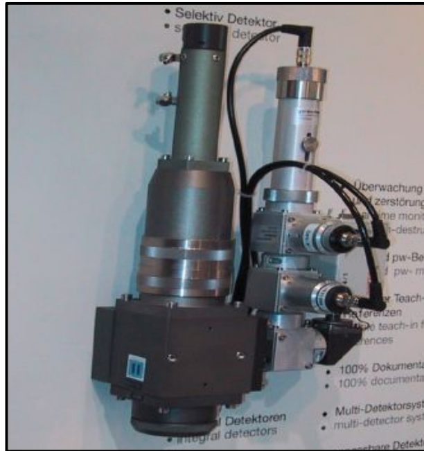
Fig. 1-2 Online welding sensor integrated on Precitec welding head
