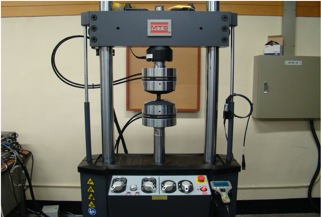
Fig. 3-3 Device configuration of tensile tester
