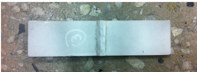
Fig. 3-5 Produced flat panel welded specimen
