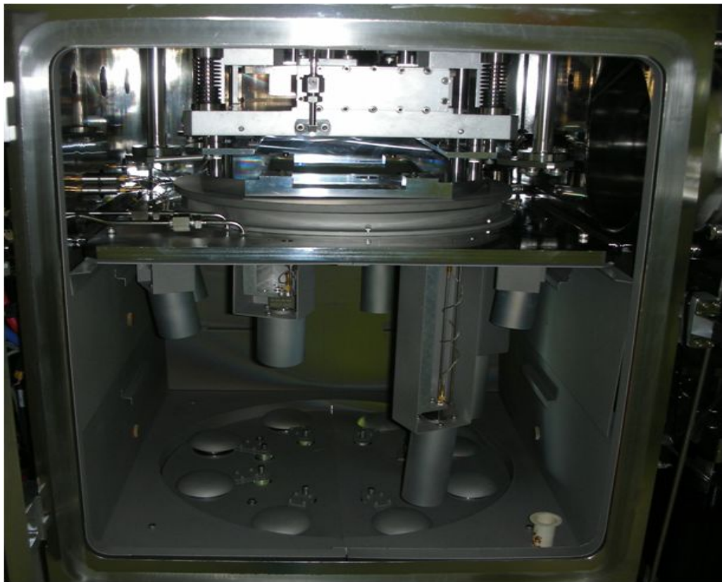
Fig. 20. Organic Evaporation Chamber (SUNIC SYSTEM plus200)
