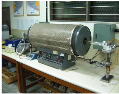
Fig. 3. 1. Horizontal tube furnace for tempering.
