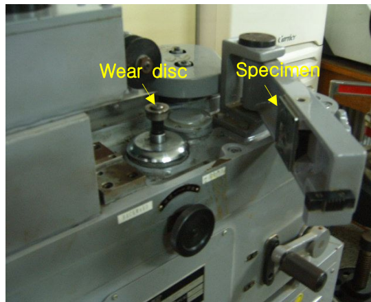
Fig. 3. 5. High speed universal wear tester.
