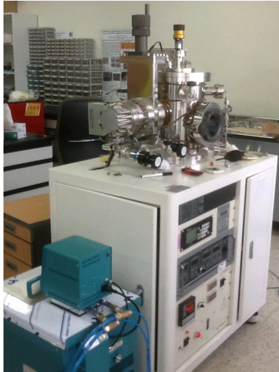
Fig .5. RF magnetron sputtering system used in this study.
