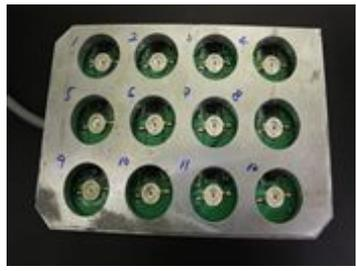
Fig. 2. Red LED module with power LED array.
