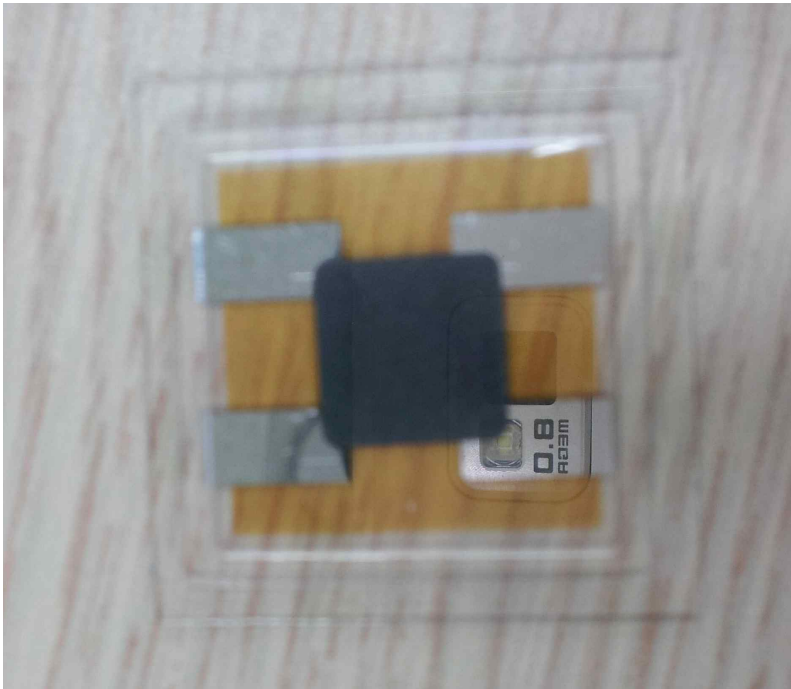
Fig. 13. manufactured OLED lighting test device
