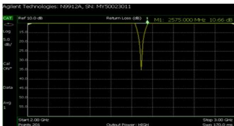
Figure 4.11 Frequency measured at -10\text{dB} , f_{\text{max}} is 2.575GHz
