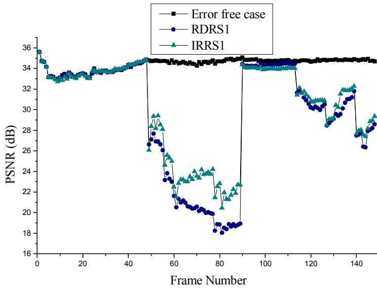
Fig. 5.3 Quality of tennis sequence with either RDRS or IRRS in erroneous network (PLR 5%).
