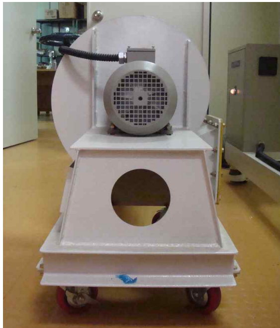
Fig. 2.14 Photograph of suction fan.
