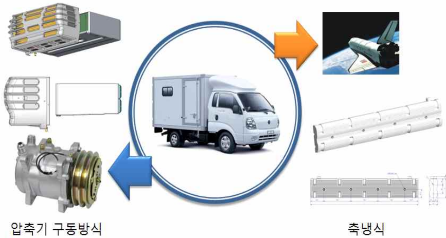
Fig. 1.1 Refrigerating system of using compress and PCM.
