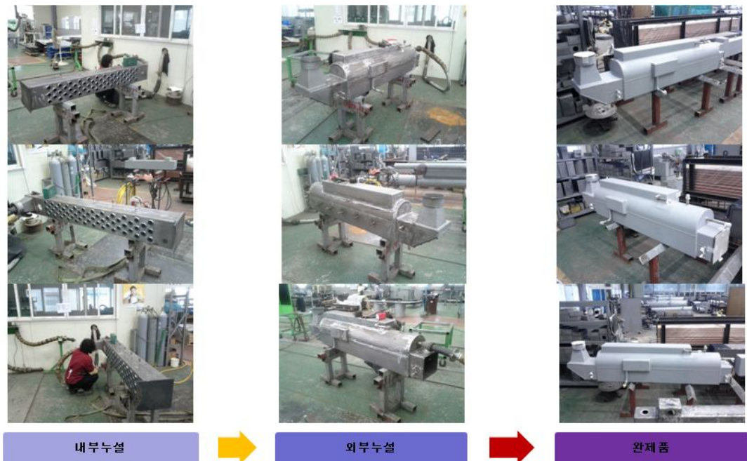
Fig. 2.9 Making process of a Lab. scale high-temperature generator.
