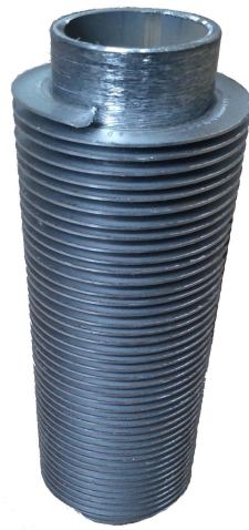
Fig. 2.4 Photograph of a finned tube.
