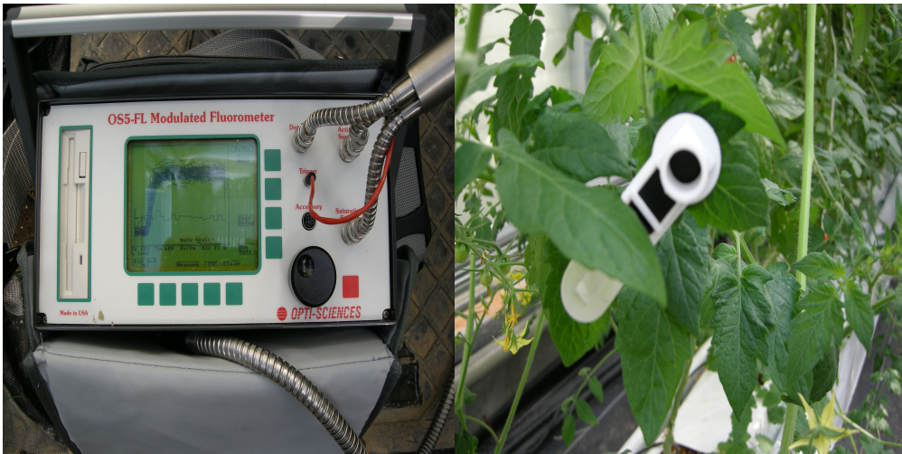
Figure 11. The portable fluorometer measurement of the tomato by the CO_2 concentration.
