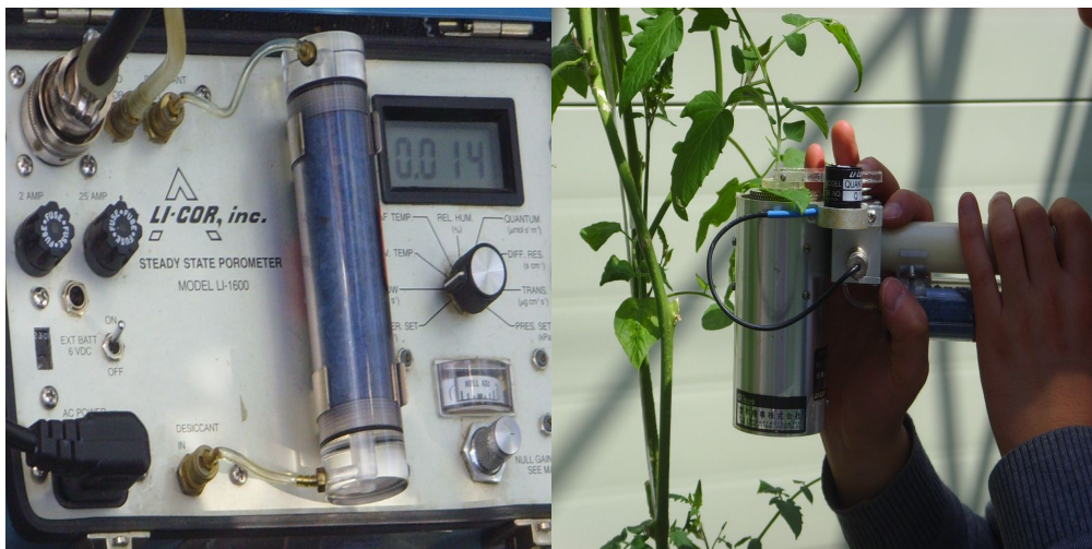
Figure 12. The portable Porometer(Li-1600, Li-Cor) measurement of the tomato by the CO 2 concentration.
