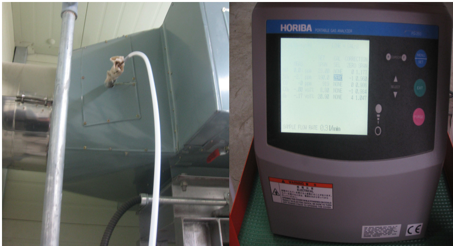
Figure 20. Pictures of exhaust gas sampling (left) and measurement (right).
