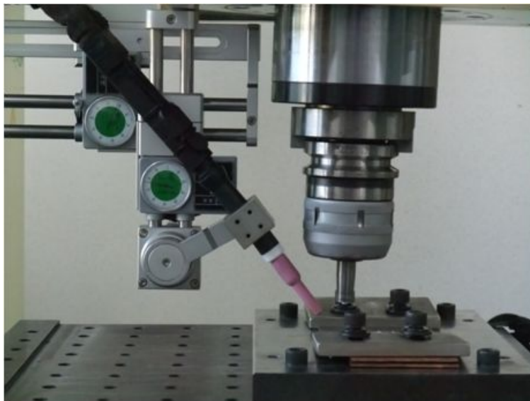
Fig. 3.2 Setup for TIG assisted hybrid FSW welding process
