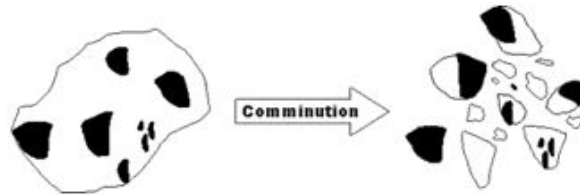
Figure 1.1. Breaking of larger materials to smaller pieces. Darker regions represent the valuable minerals. (Met-Solve,2010)
