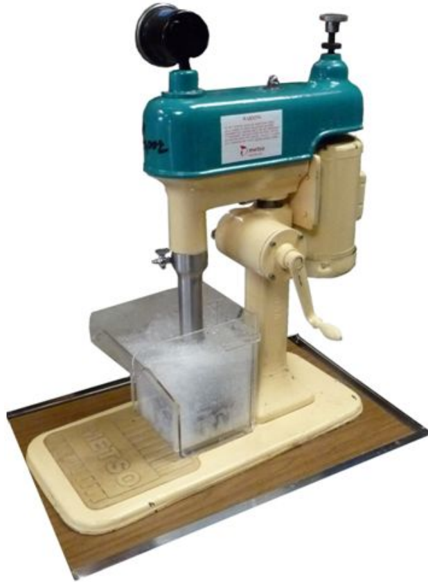
Figure 3.6 Laboratory scale Denver Sub-A type flotation machine.
