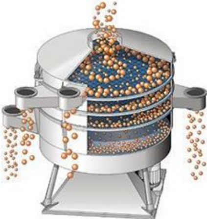
Figure 1.3. Vibratory screen with multiple removable and replaceable decks.( www.traderscity.com )
