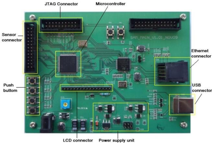
Fig 3.3 Printed circuit board of the control module.
