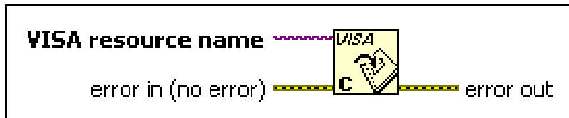
Fig 3.12 VISA Close Function in Labview.
