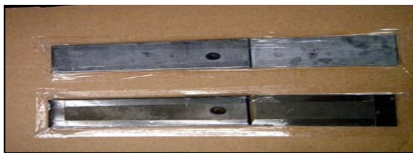
Fig.4-3 Application on NAUT of Spot welding specimen
