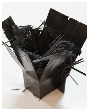
Photo. 11 Collapsed shape of CFRP hat-shaped sectional member, 2 interface (dry specimen, outer angle 0°)
