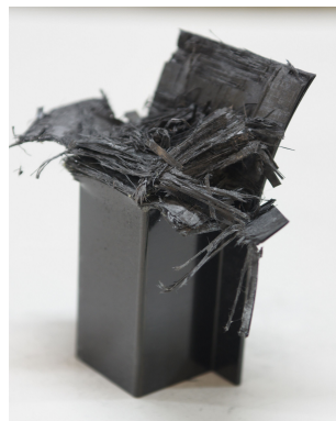
Photo. 35 Collapsed shape of CFRP hat-shaped sectional member, 0^{\circ}/90^{\circ} (wet specimen, stacking angle)
