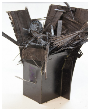
Photo. 8 Collapsed shape of CFRP hat-shaped sectional member, 4 interface (dry specimen, outer angle 90°)
