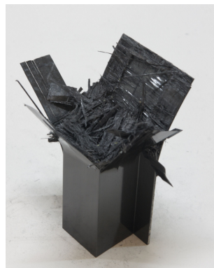
Photo. 34 Collapsed shape of CFRP hat-shaped sectional member, 90°/0° (wet specimen, stacking angle)
