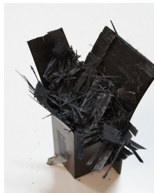
Photo. 15 Collapsed shape of CFRP hat-shaped sectional member, 7 interface (dry specimen, outer angle 0^\circ )
