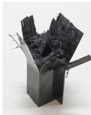
Photo. 22 Collapsed shape of CFRP hat-shaped sectional member, 3 interface (wet specimen, outer angle 0^\circ )
