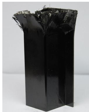
Photo. 26 Collapsed shape of CFRP hat-shaped sectional member, 15° (dry specimen, stacking angle)
