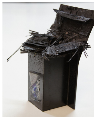
Photo. 6 Collapsed shape of CFRP hat-shaped sectional member, 2 interface (dry specimen, outer angle 90^\circ )
