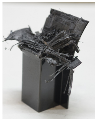
Photo. 20 Collapsed shape of CFRP hat-shaped sectional member, 7 interface (wet specimen, outer angle 90°)
