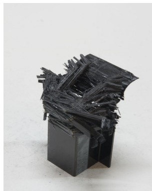
Photo. 33 Collapsed shape of CFRP hat-shaped sectional member, 90° (wet specimen, stacking angle)
