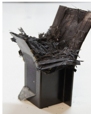
Photo. 30 Collapsed shape of CFRP hat-shaped sectional member, 0^{\circ}/90^{\circ} (dry specimen, stacking angle)
