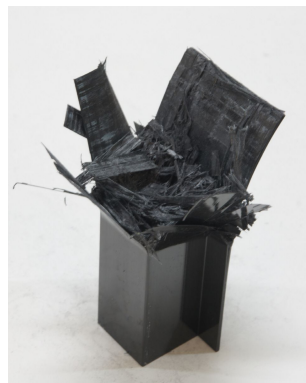
Photo. 24 Collapsed shape of CFRP hat-shaped sectional member, 6 interface (wet specimen, outer angle 0^\circ )
