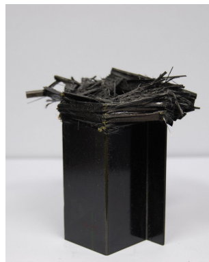
Photo. 28 Collapsed shape of CFRP hat-shaped sectional member, 90° (dry specimen, stacking angle)
