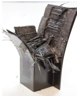
Photo. 9 Collapsed shape of CFRP hat-shaped sectional member, 6 interface (dry specimen, outer angle 90°)
