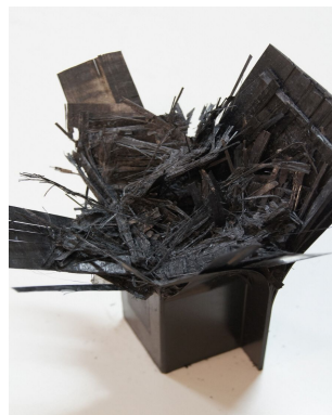
Photo. 13 Collapsed shape of CFRP hat-shaped sectional member, 4 interface (dry specimen, outer angle 0°)
