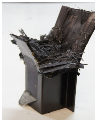
Photo. 10 Collapsed shape of CFRP hat-shaped sectional member, 7 interface (dry specimen, outer angle 90°)
