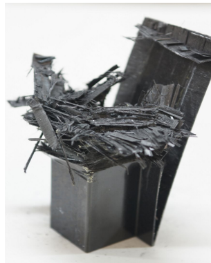
Photo. 16 Collapsed shape of CFRP hat-shaped sectional member, 2 interface (wet specimen, outer angle 90^\circ )
