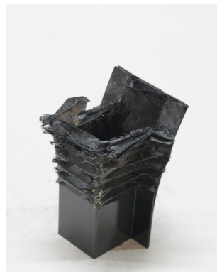
Photo. 32 Collapsed shape of CFRP hat-shaped sectional member, 45° (wet specimen, stacking angle)
