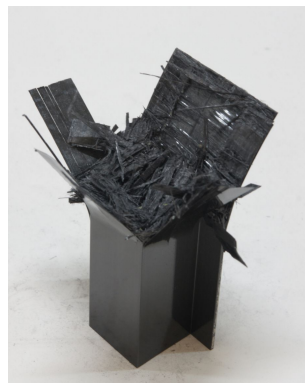
Photo. 25 Collapsed shape of CFRP hat-shaped sectional member, 7 interface (wet specimen, outer angle 0°)
