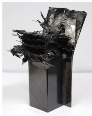
Photo. 27 Collapsed shape of CFRP hat-shaped sectional member, 45° (dry specimen, stacking angle)
