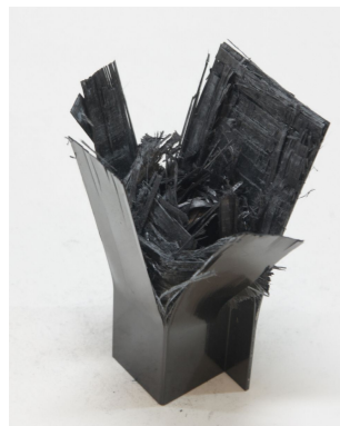
Photo. 21 Collapsed shape of CFRP hat-shaped sectional member, 2 interface (wet specimen, outer angle 0°)
