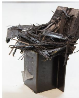
Photo. 7 Collapsed shape of CFRP hat-shaped sectional member, 3 interface (dry specimen, outer angle 90°)
