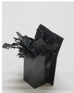
Photo. 31 Collapsed shape of CFRP hat-shaped sectional member, 15° (wet specimen, stacking angle)
