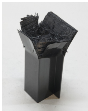
Photo. 23 Collapsed shape of CFRP hat-shaped sectional member, 4 interface (wet specimen, outer angle 0^\circ )
