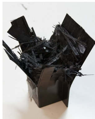
Photo. 12 Collapsed shape of CFRP hat-shaped sectional member, 3 interface (dry specimen, outer angle 0°)
