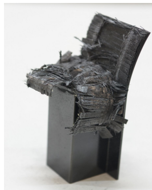
Photo. 19 Collapsed shape of CFRP hat-shaped sectional member, 6 interface (wet specimen, outer angle 90^\circ )
