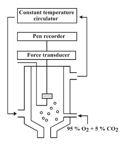
Fig. 1. A schematic representation of the recording system for isometric contraction with 15 mL tissue bath.
