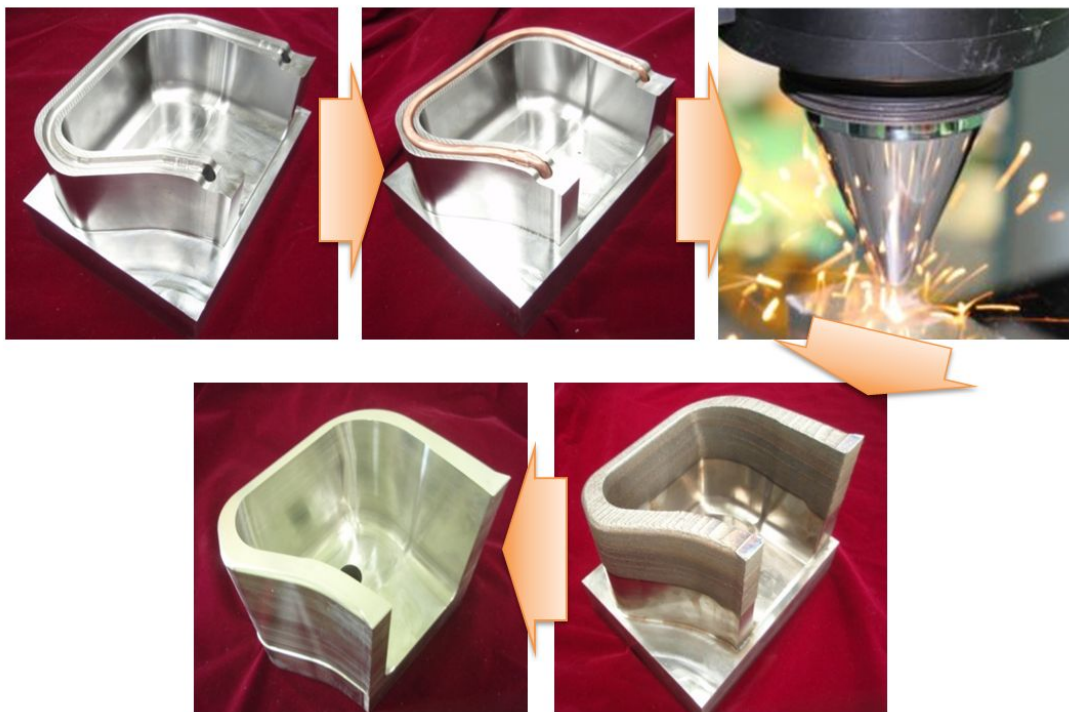
Fig. 3 Manufacturing procedure of the mould using direct metal tooling process
