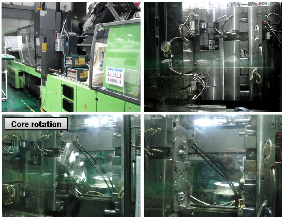
Fig. 73 Injection moulding experiments for the human-friendly computer mouse
