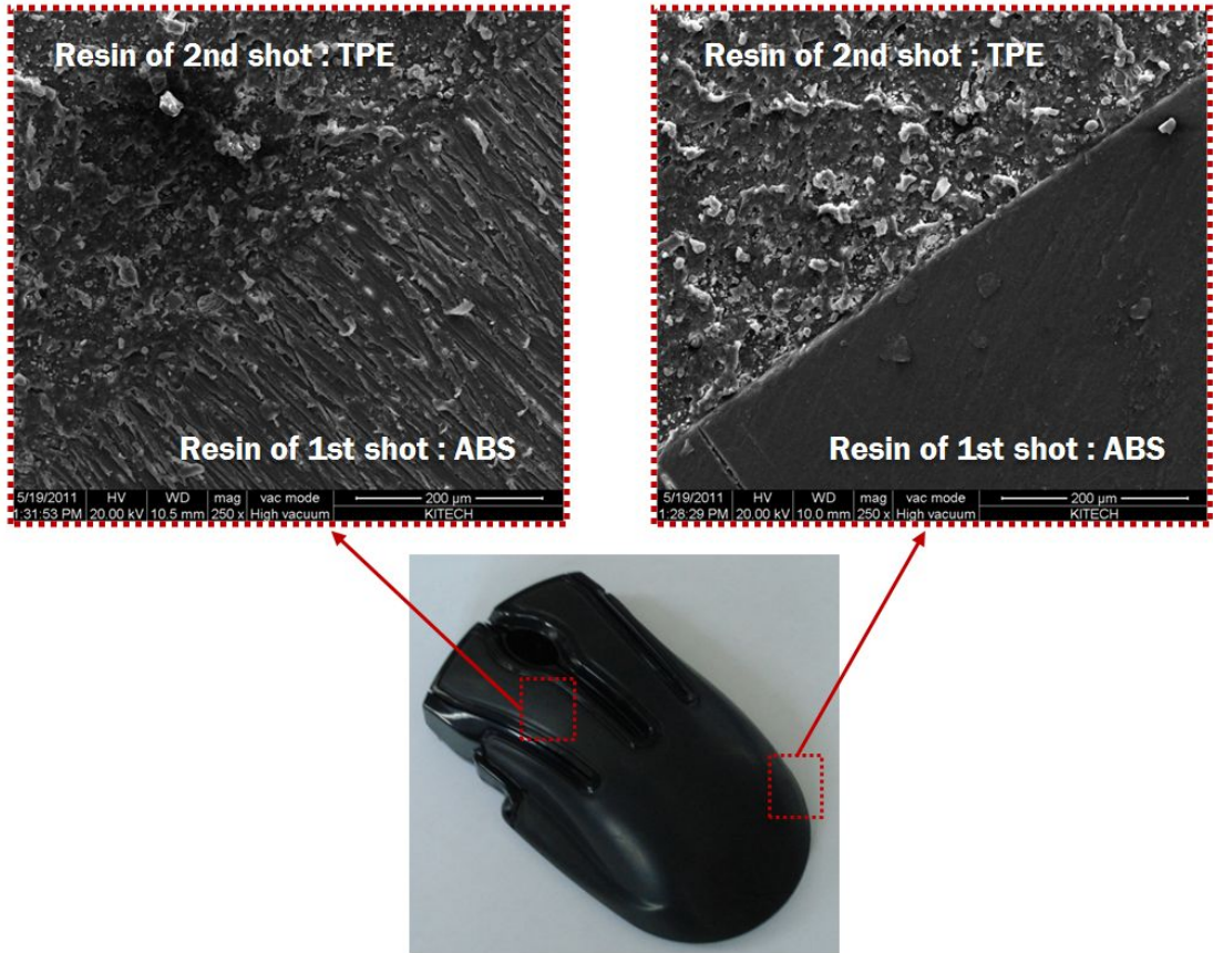
Fig. 76 Microstructure in the vicinity of the welded region (Human-friendly computer mouse)
