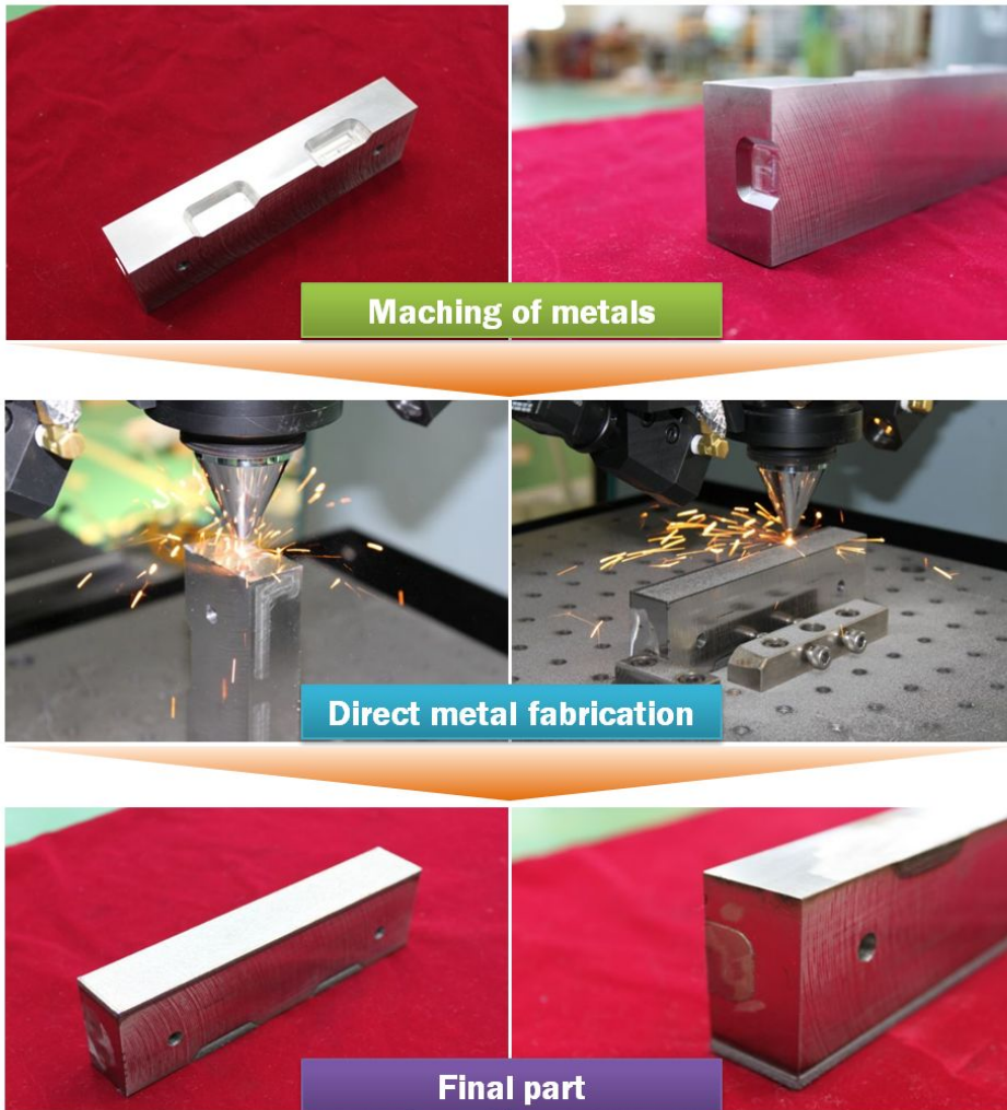
Fig. 67 Manufacturing procedure of the multi-sliced mould core with 3D conformal cooling channel using rapid tooling process
