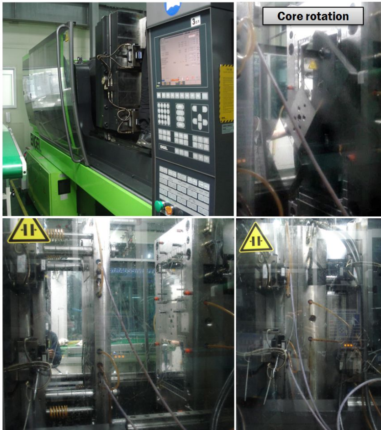
Fig. 69 Injection moulding apparatus with the multi-sliced mould set for experiments
