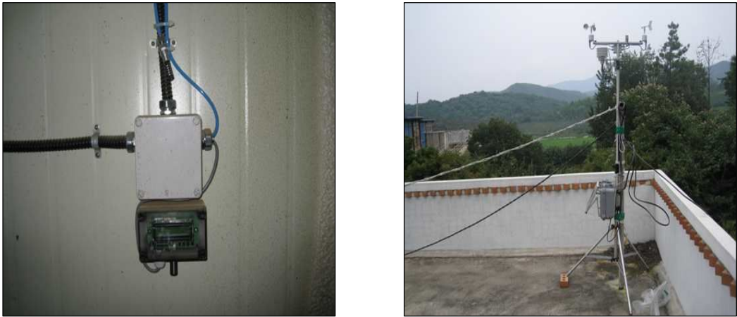
Fig. 4.16. Temperature and humidity measurement equipment for inside and outside of pig house.
