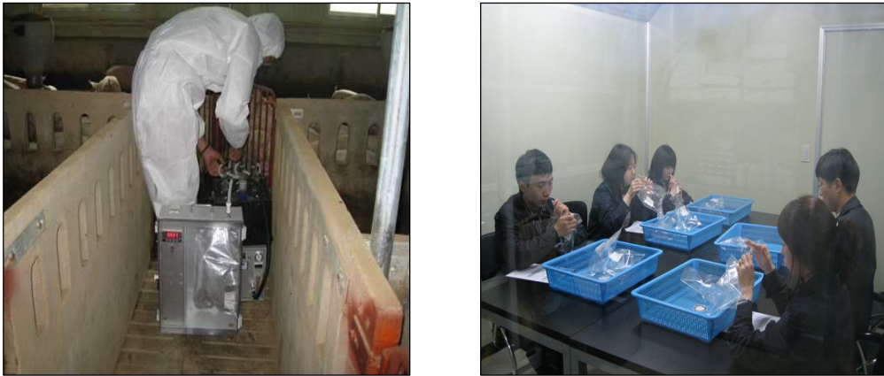
Fig. 3.1. Mixture odor measurement and analysis on the pig house.
