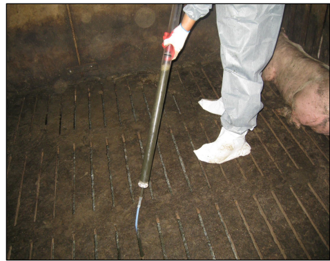
Fig. 3.6. Sampling of microorganism at pig house.
