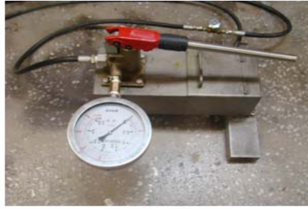
(b)Hydraulic Pump & Gauge
