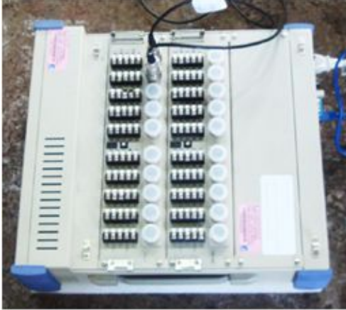
(a) Data logger for 20-channels
