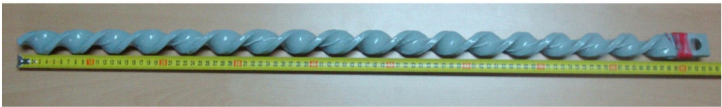
Figure 2.5 Spiral bolt making process. (a) Surface molding, (b) strain gauge attach, (c) using paint coating, (d) complete product.
