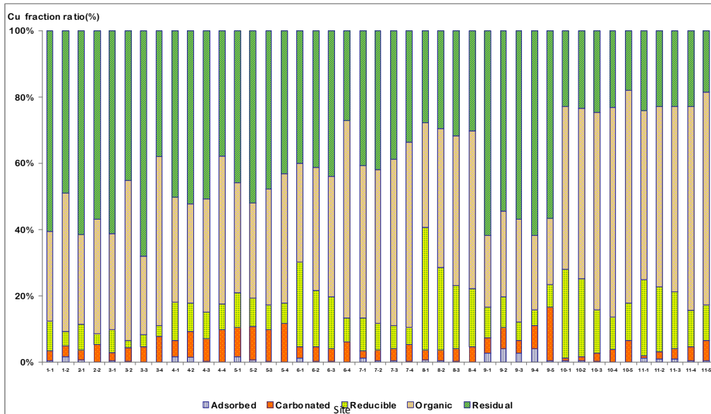
Fig. 36. The copper fraction ratio of different forms of sediments in Youngil bay.
