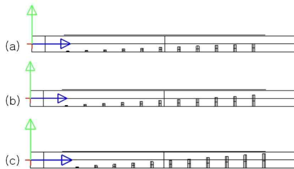
Figure 36. Slant change of slope patterns(distance 3.5 mm); (a)Slant 50 % about thickness(3 mm), (b)Slant 70 % about thickness(3 mm), (c)Slant 90 % about thickness(3 mm).
