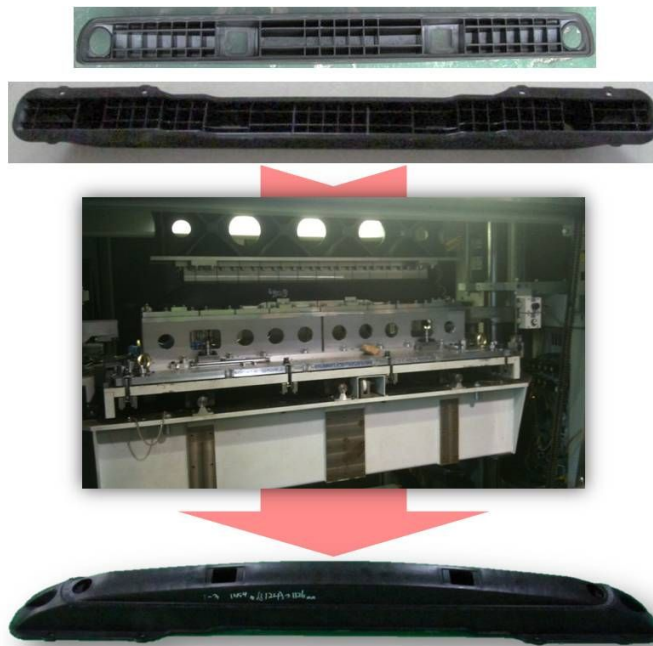
Fig. 46 Vibration welding and final product
