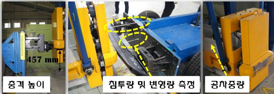
Fig. 48 Experimental set-up of low-speed frontal collision test
