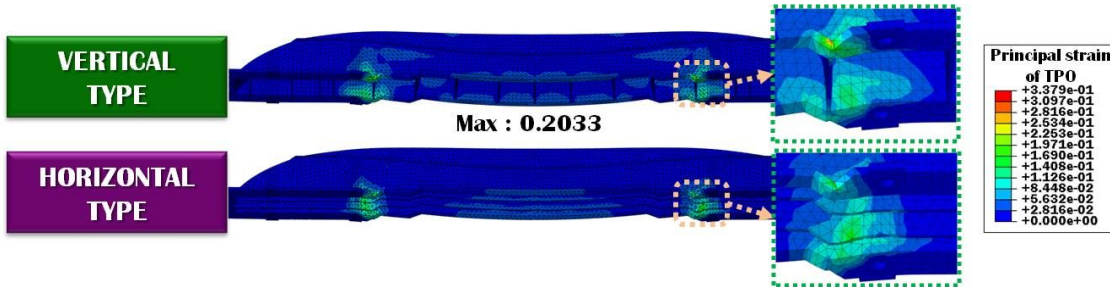
Fig. 36 Variation of principal strain distributions for ribs direction
