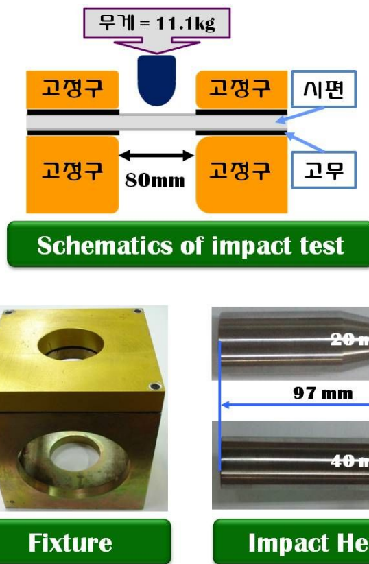
Fig. 7 Schematics and experimental devices for stretching type of impact test
