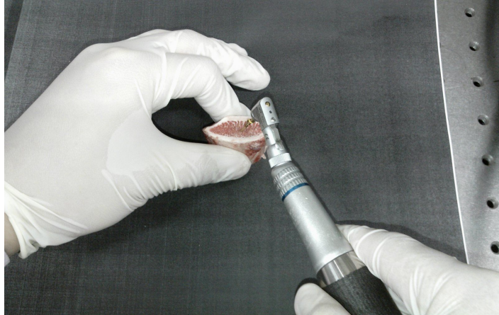
Fig. 3-17 Drilling into cow bone using Freehand method
