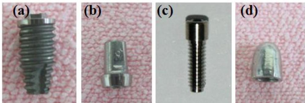
Fig. 1. Photographs of fixture, abutment and abutment screw. (a) fixture, (b) abutment, (c) abutment screw and (d) metal cap for fatigue test.
