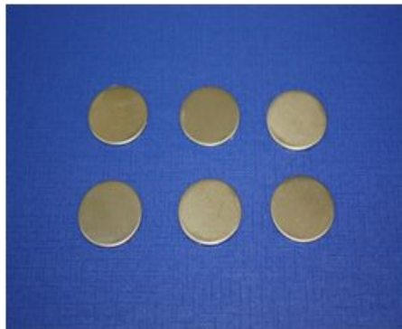
Fig. 2. Titanium disk after mechanically polishing.
