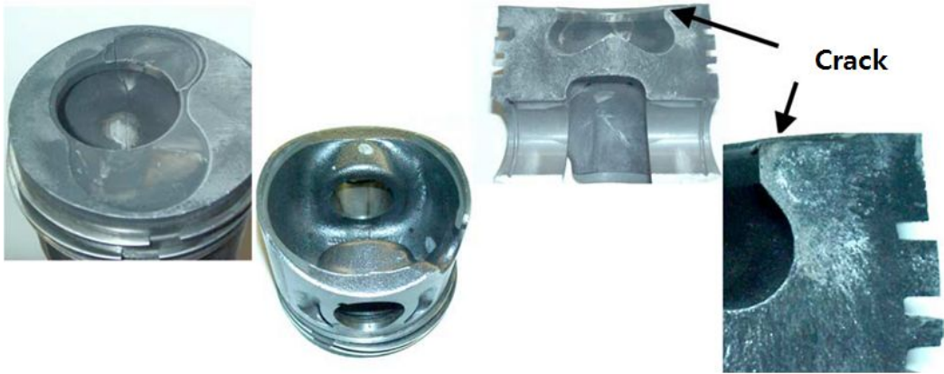
Fig. 2-4 Diesel engine piston with a crack from one side of the pin hole to the other pin hole going through the head of the piston
