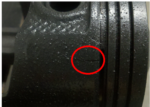
Fig. 5-2 Cracks from impact
