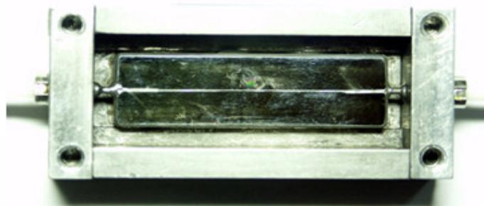
Fig. 11. Picture of PBF gas Sensor
