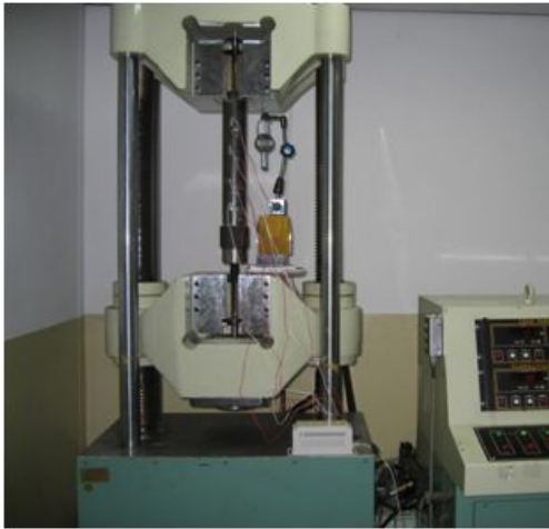
Figure 7.1 Laboratory pull-out test.
