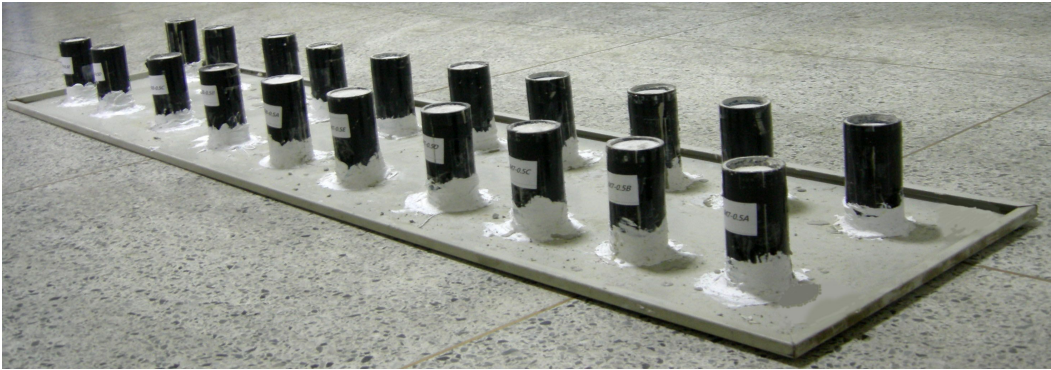
Figure 5.5 Curing of cylindrical specimens for uniaxial compression test.
