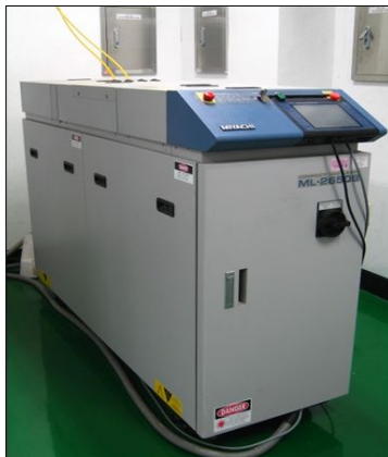
(b) Equipment and specifications of Nd:YAG Laser system
