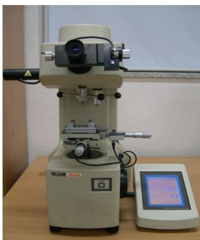
Fig. 4.8 Vickers hardness test machine and specimen
