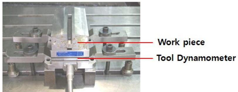
Photo. 3.2 Installation of tool dynamometer and material processing
