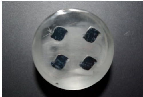
Photo. 4.3 Mounting of AlTiN layer
