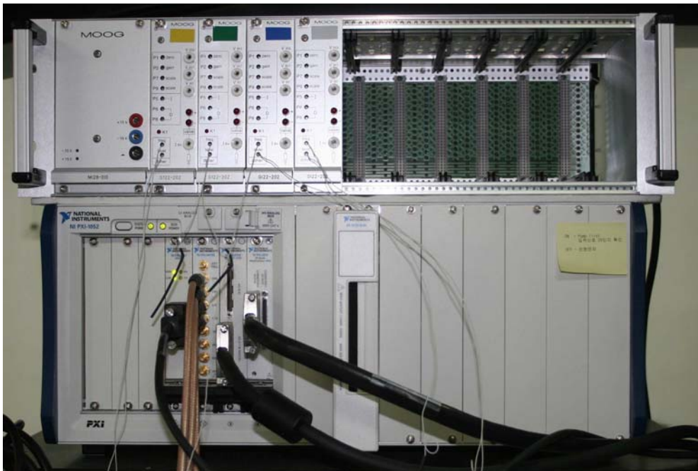
Photo. 2.3 Servo controller and signal processing unit of 4-axis hydraulic simulator.
