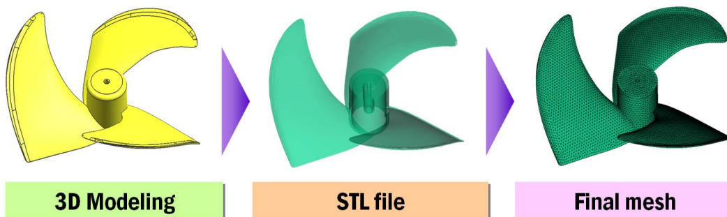
Fig. 7 Procedure of mesh generation of a plastic fan part
