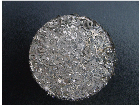
Fig. 3.3 Compaction of Ti scrap
