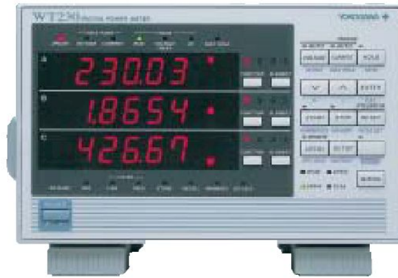
Fig. 2.17 Photograph of power meter.
