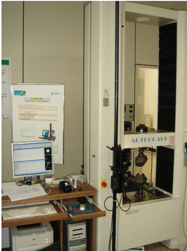
Photo. 5 Uni-axial tensile test machine SHIMAZU AG-IS 50kN
